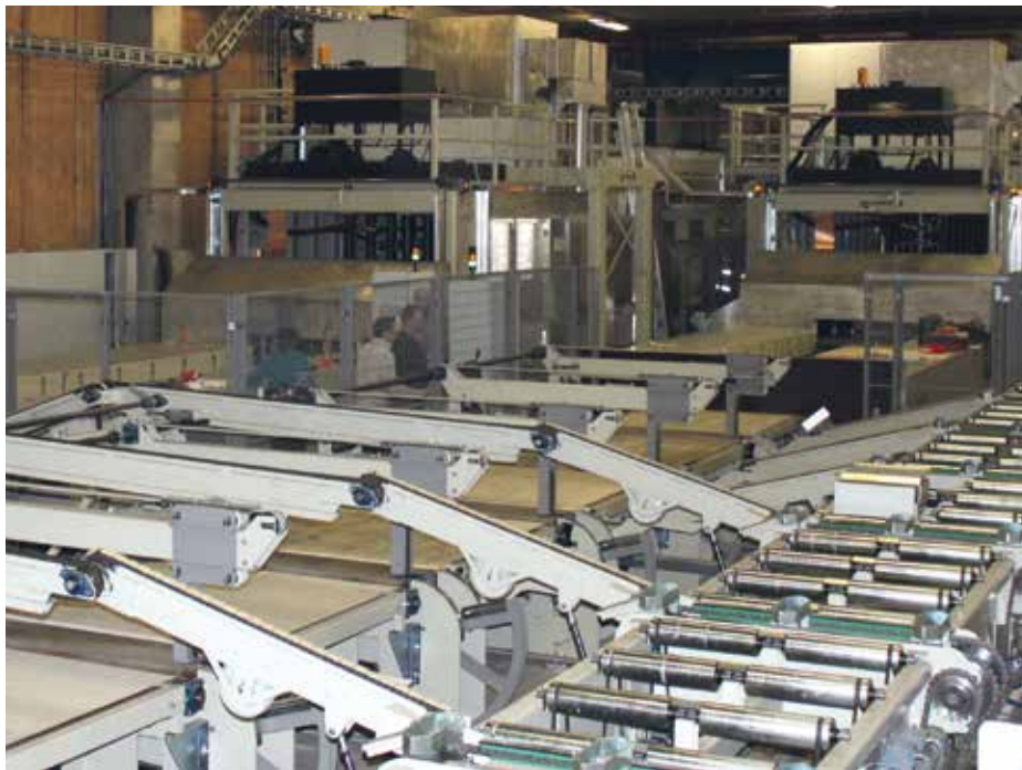
Technology cores off the new plant for laminated and glued beams at the location Imst are the two high-performance high-frequency presses.
