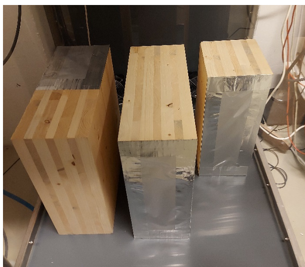
Figure 1: The sample 500038_21 in the 1 m 3 emission chamber
