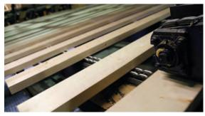
Sawn timber is graded visually on high-performance grading machines by continuously trained personnel supported by modern scanner technology immediately after cutting. Dimensions are always packaged according to thickness, width, length and quality.
